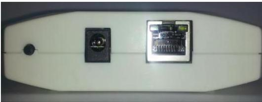
The Ethernet port (right hand of the picture) must be connected to your internet high speed connection router. No additional bridges or routers are required. The modem should have “line of sight” to the tank sensor transmitter and should not exceed 250ft of distance.
